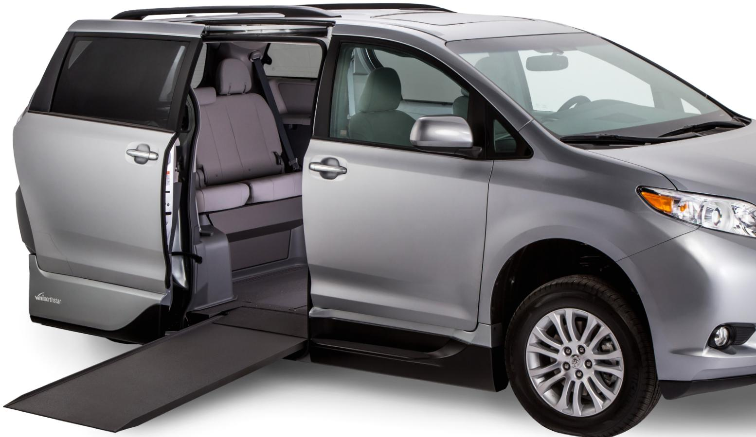
VMI prides itself in producing the easiest to use, most accessible mobility solutions in the world. The Northstar in-floor ramp system, a VMI specialty since 1993, offers an array of accessibility features that simply cannot be matched by vehicles with fold-out ramps. VMI Northstar owners get all of the benefits of an in-floor ramp without the compromise associated with rear-entry or fold-out conversions.
